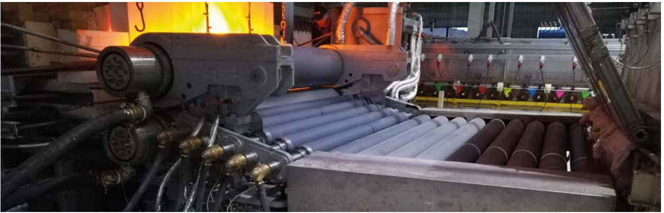
Main roller- \phi 460 mm
