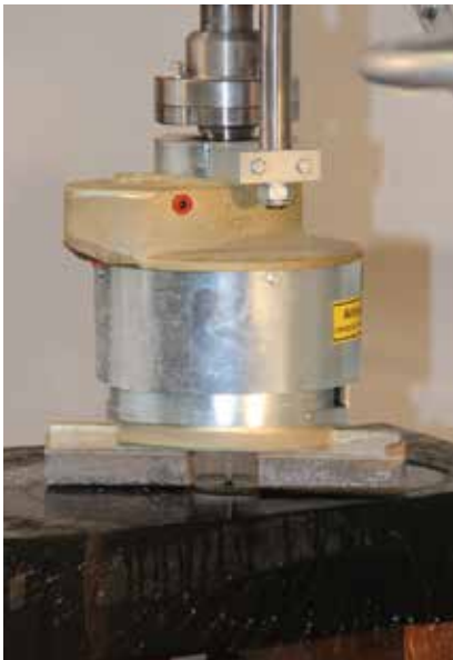
Flächenschleifen von Granit Surface polishing of granite
