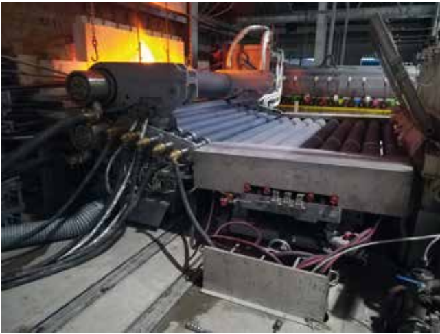
Main roller- \varnothing 460 mm
